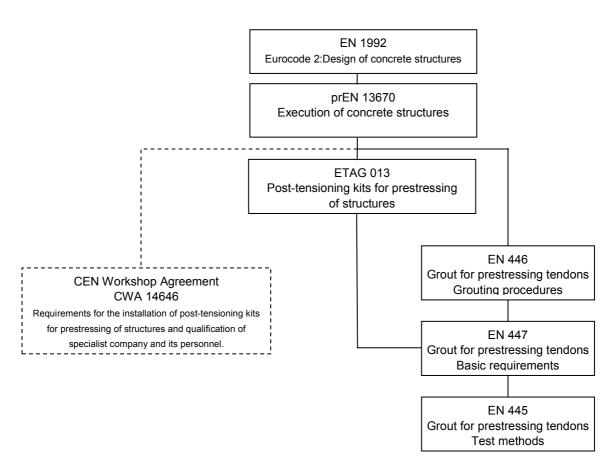
System of CEN and EOTA documents as basis for design, execution and materials selection for protective measures of prestressing systems (only main modules).
