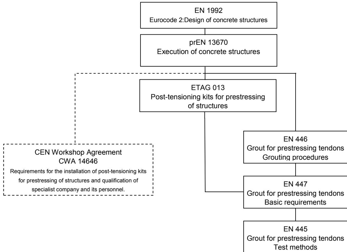
System of CEN and EOTA documents as basis for design, execution and materials selection for protective measures of prestressing systems (only main modules).
